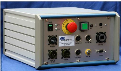
Solo standalone controller and power supply unit for the accelerator robot
