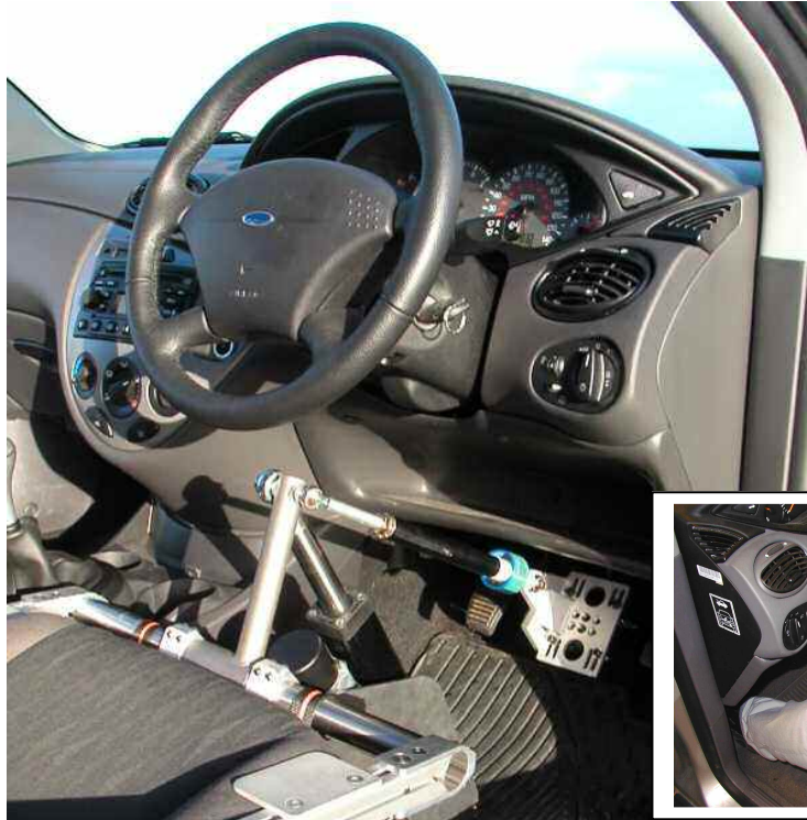
Brake robot installed in a Ford Focus. (Inset shows prototype unit with driver)
