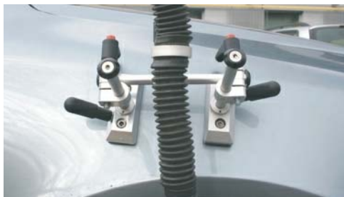
Torsion mounting assembly with magnetic holder
