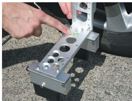
For easy adjustment of the sensor, the top of the mounting plate is fitted with a liquid level indicator.
