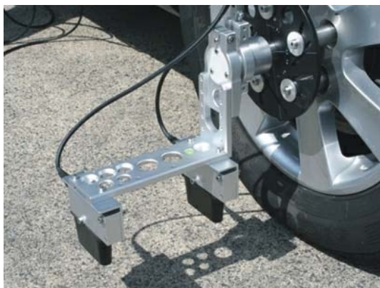
A properly mounted DCA System with two HF-xxxC Sensors
