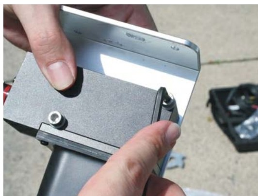
Securing the SFII-P Sensor to the mounting plate for SF Sensors on DCA mounting bracket.
