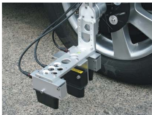
For measurement of tire slip angle, the DCA System can be fitted with an optional CORREVIT® SFII-P Sensor.
