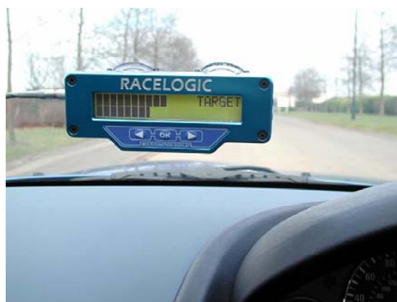
Target screen showing 0.5g decel target
